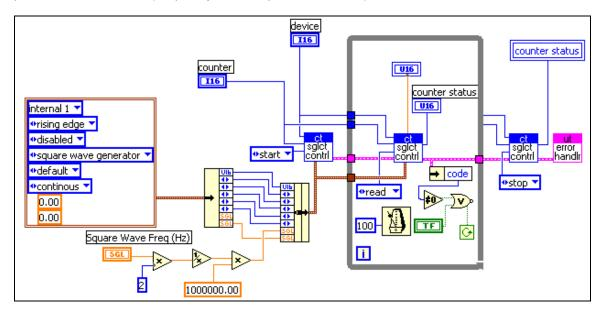
The names of the eight values within the bundle are, in top to bottom order: clock, clock edge, gate, mode, output, pulses, period and onCount.
